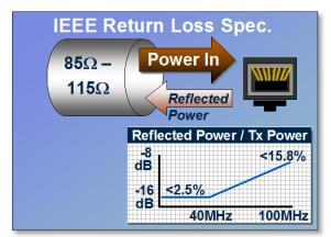
Figure 1.13 IEEE 802.3 Return Loss Specification
