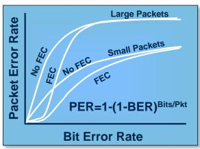
Figure 1.5 Packet Error Rate vs Bit Error Rate
