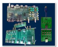
Figure 1.2 Ethernet PHY Test Fixtures
