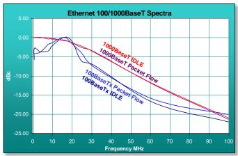
Figure 1.6 100BaseTx and 1000BaseT Transmission Spectra
