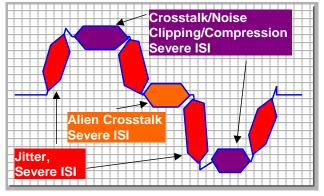
Figure 1.9 Sources of Residual Distortion
