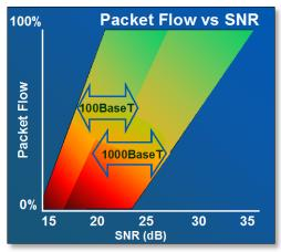
Figure 1.10 SNR vs Packet Flow
